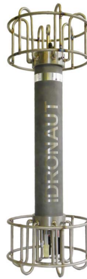
Figure 6.3: multiparametric Idronaut mod. 316 Plus probe used for the in situ measurements.
