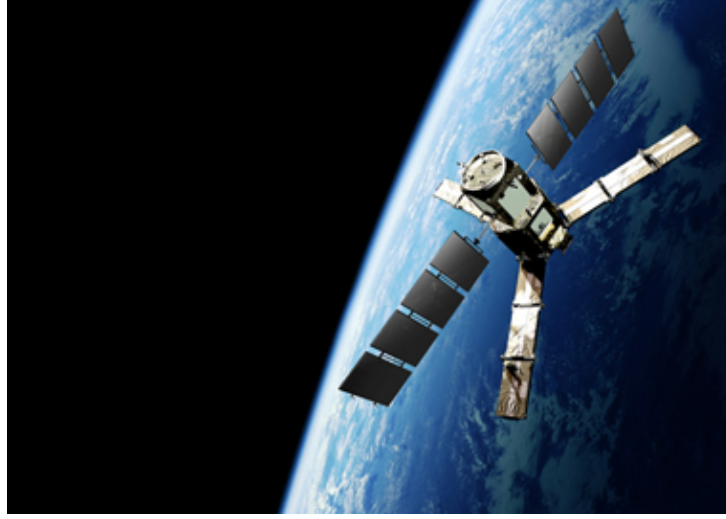
Figure 1.18: The new ESA satellite SMOS for measuring sea surface salinity and soil moisture
