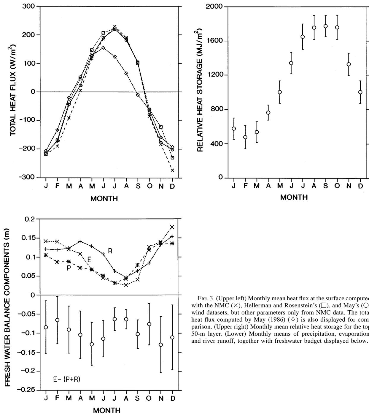
FIG. 3. (Upper left) Monthly mean heat flux at the surface computed with the NMC ( $\times$ ), Hellerman and Rosenstein's ( $\square$ ), and May's ( $\circ$ ) wind datasets, but other parameters only from NMC data. The total heat flux computed by May (1986) ( $\diamond$ ) is also displayed for comparison. (Upper right) Monthly mean relative heat storage for the top 50-m layer. (Lower) Monthly means of precipitation, evaporation, and river runoff, together with freshwater budget displayed below.
