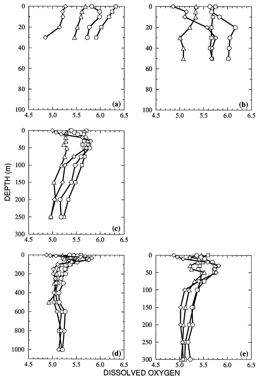
FIG. 9. Climatological profiles of dissolved oxygen ( $\text{ml l}^{-1}$ ) for (a) the northern Adriatic with bottom depth less than or equal to 50 m, (b) northern Adriatic with bottom depth greater than 50 m, (c) middle Adriatic, (d) southern Adriatic for the entire water column, and (e) southern Adriatic for the upper 300 m. Symbols indicate winter ( $\square$ ), spring ( $\circ$ ), summer ( $\diamond$ ), and autumn ( $\triangle$ ).
