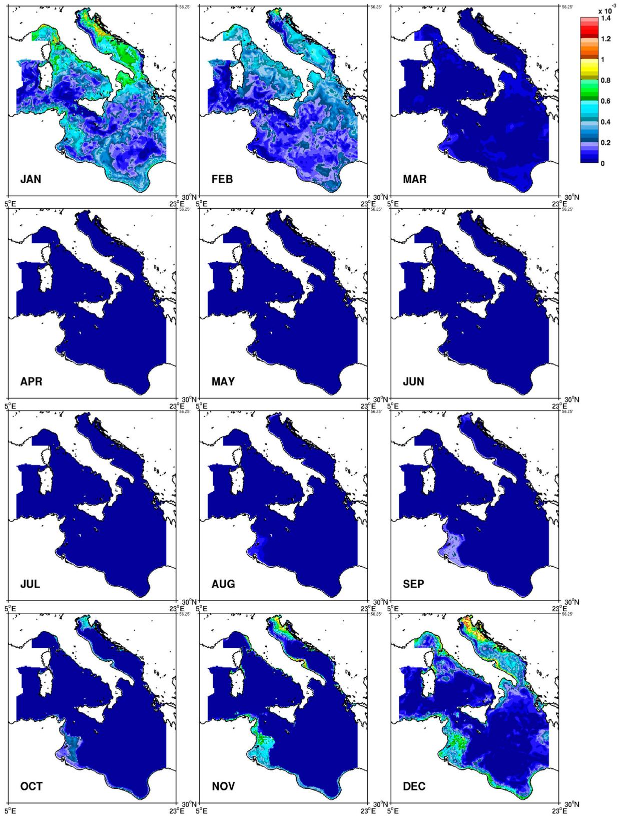
**Figure 7.** Monthly horizontal distribution of the first 100 m averaged vertical mixing coefficient calculated from Equation (2).
