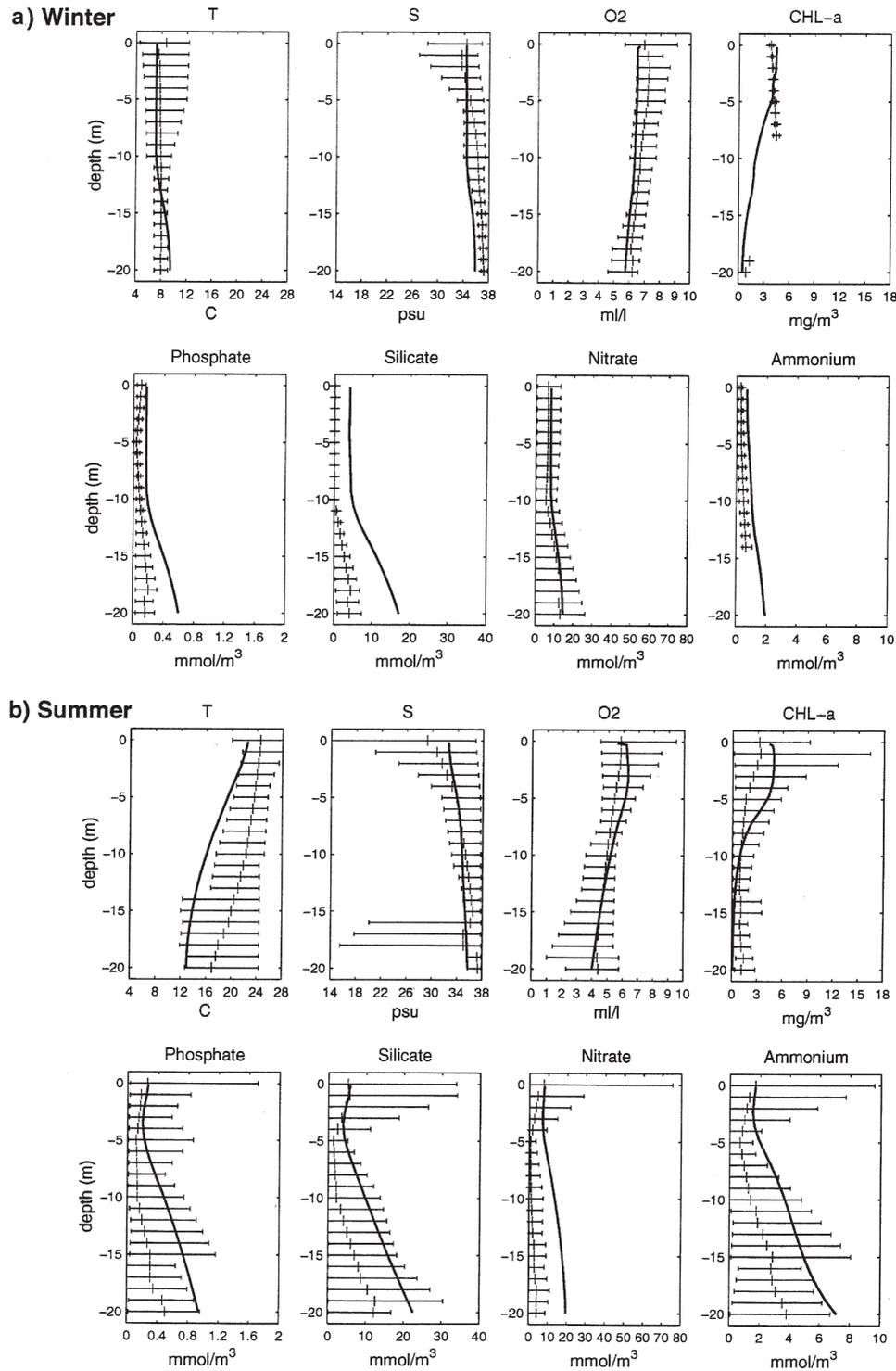
Fig. 5. Model and data comparison in winter (a) and summer (b). The continuous line is the modelled seasonal mean and the climatological observational means are shown with the range of variability (interval between maximum and minimum values found in the observations).
