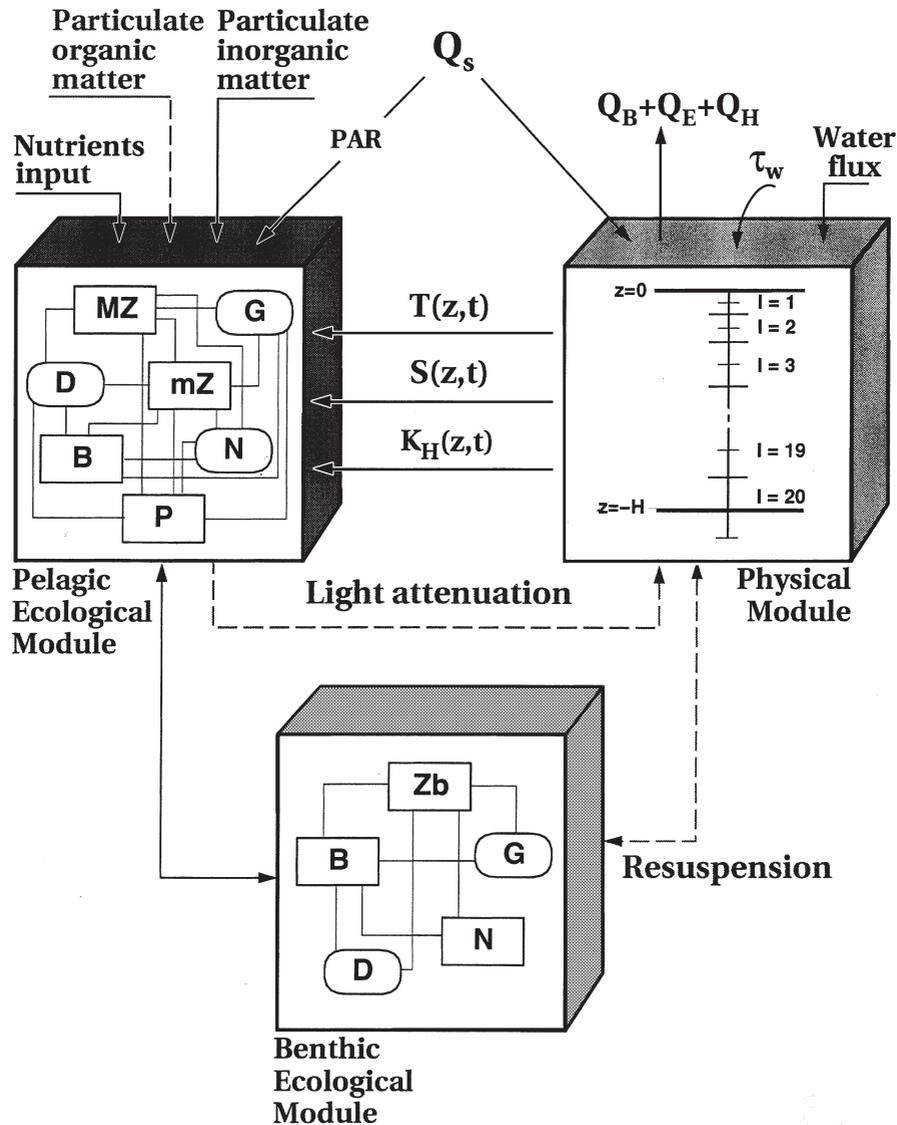
Fig. 2. Schematic description of physical and biogeochemical models, general interactions and sub-models. The dashed arrows represent forcing and interactions not yet implemented in the model. Explanation of flow diagram symbols: P = phytoplankton, MZ = mesozooplankton, mZ = microzooplankton, B = bacteria, D = organic matter (POM + DOM), G = dissolved gases, N = nutrients, Zb = Zoobenthos (after Baretta et al., 1995).
